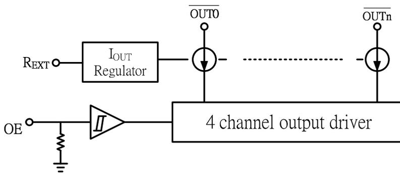
**Equivalent Circuits for OE Input**
